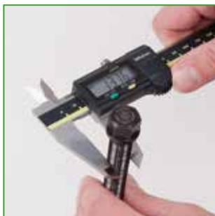
a Measure the spindle diameter.
