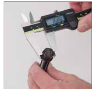
d Measure the hexagon of the spindle head.
